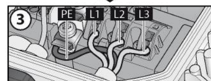
Fig. 4: Connecting wires to terminals
